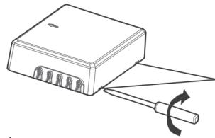
Using a flat-head screwdriver, insert the two marked positions and gently rotate the screwdriver to open the cover.
