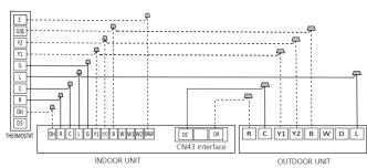
S4-2 Default on, DH function off, Turn switch off to activate DH function.
