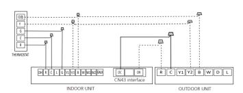
Wiring for 2H and 1C thermostat
