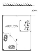
Front view of the indoor coil clearance (including air duct)
