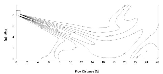
**EZPRO-18-HP-WMAH-230D-O:** Heating (Indoor:  $68^{\circ}$ F / $20^{\circ}$ C Outdoor:  $44.6^{\circ}$ F / $7^{\circ}$ C) Discharge angle  $84^{\circ}$
