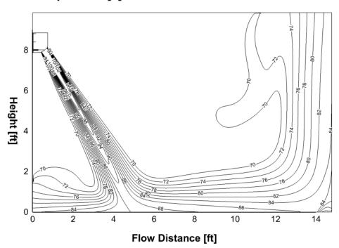
**EZPRO-18-HP-WMAH-230D-O:** Cooling (Indoor: 80.6°F /27°C Outdoor: 95°F /35°C) Discharge angle 50°
