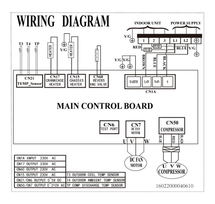
Outdoor unit wiring diagram: 16022000040790
