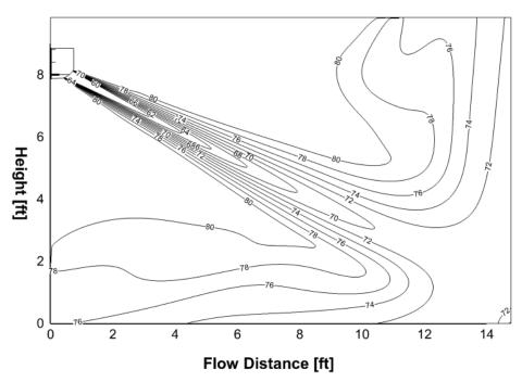
**EZPRO-09-HP-WMAH-115D-O:** Heating (Indoor: 68°F /20°C Outdoor: 44.6°F /7°C) Discharge angle 90°
