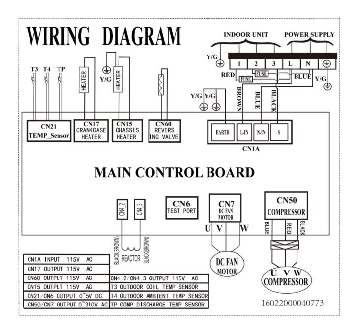
Outdoor unit wiring diagram: 16022000040610
