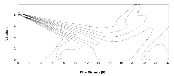
**EZPRO-24-HP-WMAH-230D-O:** Heating (Indoor: 68°F /20°C Outdoor: 44.6°F /7°C) Discharge angle 77°
