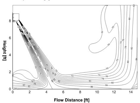
**EZPRO-12-HP-WMAH-115D-O:** Cooling (Indoor: 80.6°F /27°C Outdoor: 95°F /35°C) Discharge angle 58°
