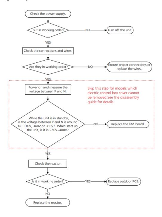
**TS11-S-INV:** Compressor top (or IPM) temp. Protection diagnosis and solution **Description:** If the temperature of the IPM module is higher than a certain value the LED displays a fault code.
