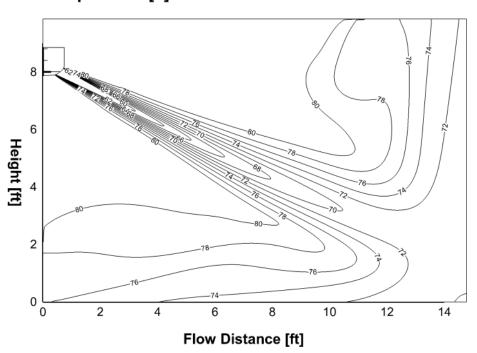
**EZPRO-12-HP-WMAH-115D-O:** Heating (Indoor: 68°F /20°C Outdoor: 44.6°F /7°C) Discharge angle 90°
