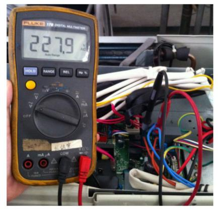
2. Turn the power off and use a digital tester to measure the resistance. The value should be 1.8~2.5  $K\pm5\%\Omega$ .
