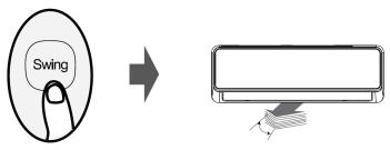
When the Swing button is continuously pressed, five different airflow directions can be set. The louver will move to a different range each time the button is pressed. Press the button until the preferred direction is reached.
