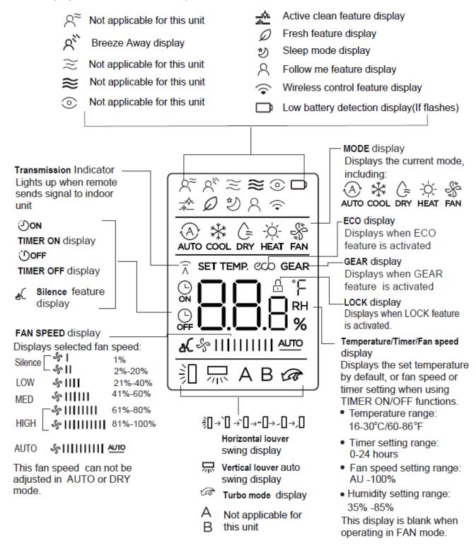
All indicators shown in the figure are for the purpose of clear presentation. But during the actual operation, only the relative function signs are shown on the display window.
