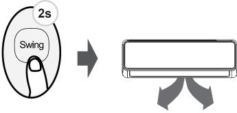
When this button is pressed for more than 2 seconds, the vertical louver swing function is activated.
