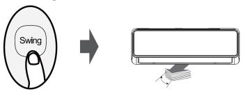
The horizontal louver will swing up and down automatically when pressing the Swing button. Press again to make it stop.
