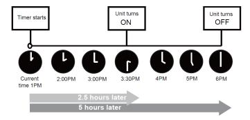
Example: If current time is 1:00pm, the unit will turn on 2.5 hours later (3:30pm) and turn off at 6:00pm.
