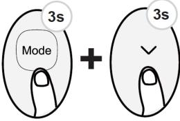
Press the Mode button and arrow down button simultaneously for more than 3 seconds to activate this function. The remote will display "F2". When setting the panel status, press the up or down arrow buttons of the remote control to control the rise or fall of the grille. Press any other button to exit the setting.
